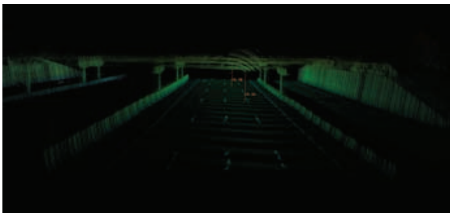
Figure 3. Bridge height measurement taken with Mandli data collection vehicle. Note lane markings visible along with road signs.
