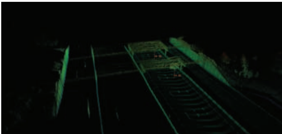
Figure 4. Bridge height and other infrastructure position measurements are accurately determined even with the vehicle travelling at full road speed.
