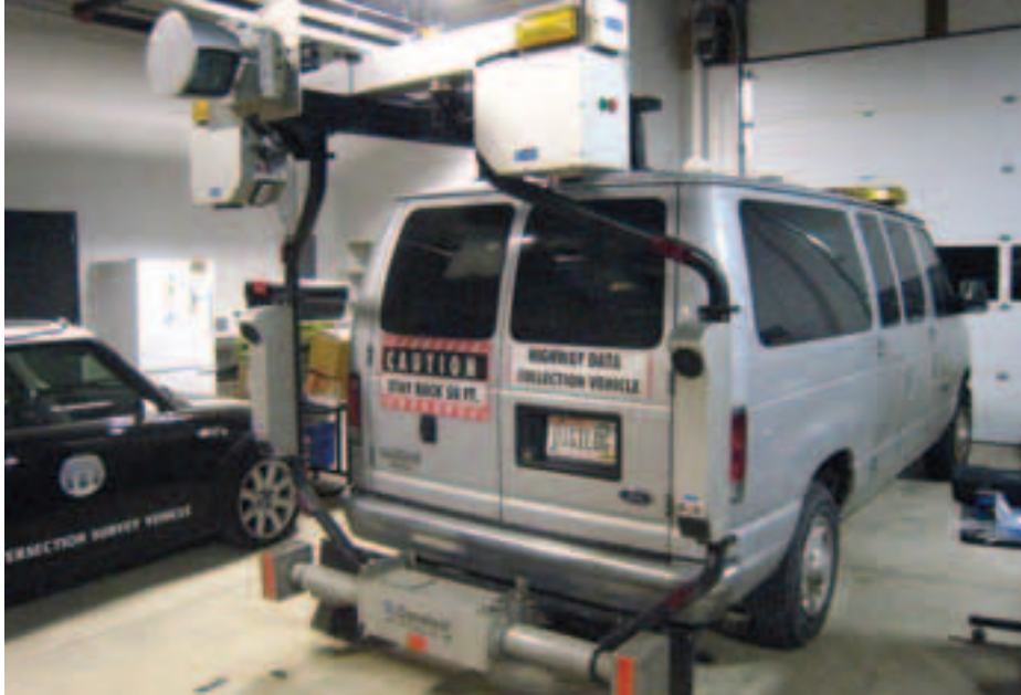
Figure 2. Mandli Data collection van equipped with LIDAR sensor.
