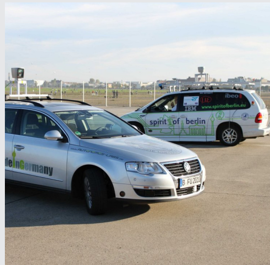
Figure 2: A driverless car. The Spirit of Berlin is an autonomous car based on the HDL-64E sensor, designed by the Artificial Intelligence Group at the Freie Universität Berlin in 2007. Picture courtesy: AutoNOMOS Project.
